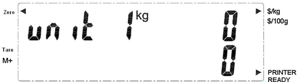
2. Select pricing unit by pressing **[1]** ~ **[2]**. The scale backs pricing mode. The symbol "◀" displays in **Unit Weight**.
