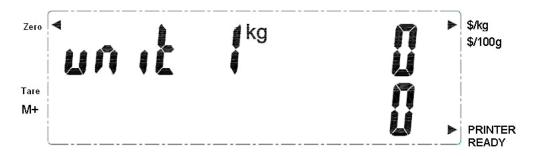
Select pricing unit by pressing 1 ~ 2. The scale backs pricing mode. The symbol " <sup>4</sup> " displays in Unit Weight.
